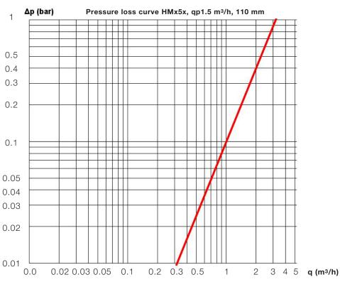
Δp Loss of pressure in bar q Flow rate in m³/h
