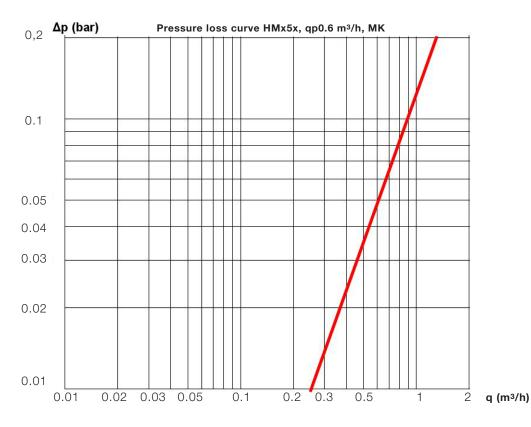
$\Delta p$  Loss of pressure in bar  $\,$  q Flow rate in  $m^3/h$
