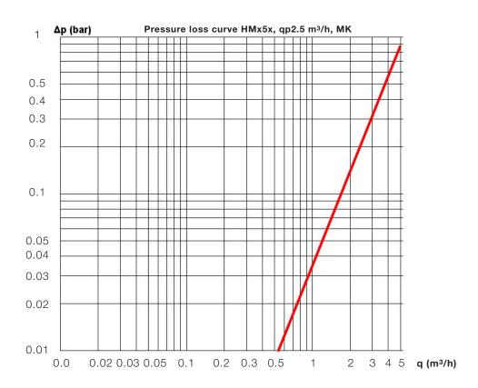
Δp Loss of pressure in bar q Flow rate in m<sup>3</sup>/h
